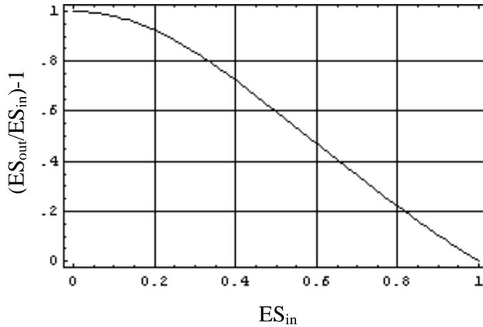
Figure 2 is a plot of  $(ES_{out}/ES_{in})-1$  versus  $ES_{in}$  for a simple 2x bias amplifier. This illustrates the relative loss of effectiveness of the bias amplifier as effect size increases. Above an  $ES_{in}$  of about 58%, which is equivalent to a hit rate of 79%, the amplifier becomes relatively inefficient. PRD data is always statistically distributed, and while this
